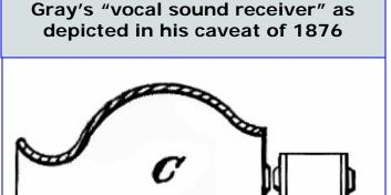
the rub" ([9], p. 197). Soon after, he instructed his instrument maker, William Goodridge, to construct a liquid transmitter, as described in his caveat [31], and in July 1876, Gray tried it out using one of his octoplex "wooden sounding box" receivers. Obviously, the test failed and could not have done otherwise, since the receiver he utilized was absolutely unsuitable for receiving (wideband) vocal sounds, because it was tuned to a single tone.
